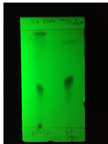
Figure 1: On left bipyridine and terpyridine mixture and on right bipyridine standard in 4:6 ethyl acetate and hexane and 1 drop of ammonium hydroxide
